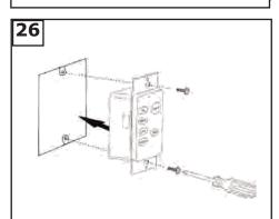
Install wall control unit to outlet box using machine screws provided.
